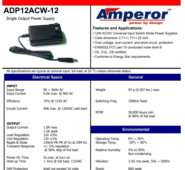
**OVP** Protection OCP protection 4A max. Short circuit protection Auto-Restart Mode
